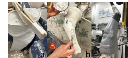
Figure 3 ■ a) A stifle cast that has been sealed and filled with liquid plaster. b) A certified prosthetist modifies the plaster positive of a stifle cast. They strategically apply plaster to create space where needed, and remove it over load-tolerant areas. c) The lamination of layers of fibreglass and resin to create a stifle brace. (Images provided courtesy of PawsAbility)
